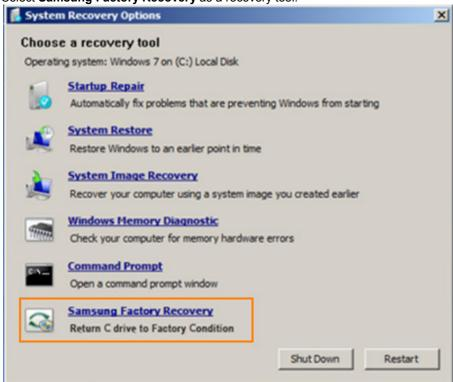
4. The system will be restored to the default factory settings. The recovery will be performed automatically. It will take about 10 minutes to recover the system. After the recovery, the system will automatically restart.
