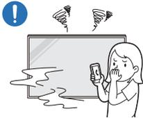
If the product generates a strange noise, a burning smell, or smoke, unplug the power plug immediately and contact your Samsung Customer Service Centre.
