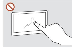
Do not scratch the screen with nails or sharp objects. Scratches may leave marks or damage the product.
