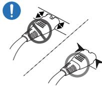
When connecting the power plug to the port, be sure to connect it completely.
