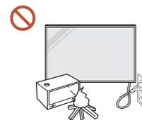
Do not install the power cable (DC power supply) and the product near head sources.
