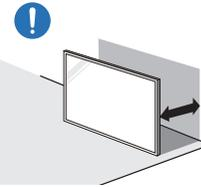
When installing the product, keep it at a distance from the wall so that it is well ventilated.
