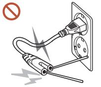
While the power plug is plugged into a power socket, do not insert a chopstick or other conductor into a remaining power socket. Also, after disconnecting the power plug from the power socket, do not touch the pins of the plug immediately.
