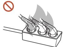
**Do not connect multiple products to a single power socket.**
