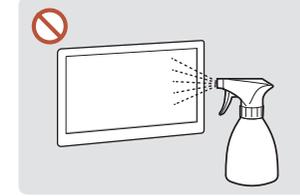
Do not spray water directly on any part of the product. Product failure, an electric shock or fire may result from water that enters the product.
